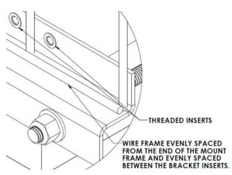
a. If two wire cages are provided, align the cages to be between one set of the threaded inserts as illustrated below.
